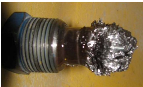
830E front wheel hub MAG-PROBE® captures material indicating impending bearing failure. The use of this Probe saved the Hub & Spindle from damage.
