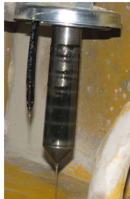
MAG-PROBE® 830E wheel motor sump filler cap after 486 hours of normal operation.
