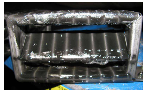
MAG-SHIELD® installed in an 830E wheel motor sump after 2026 hours of normal operation.
