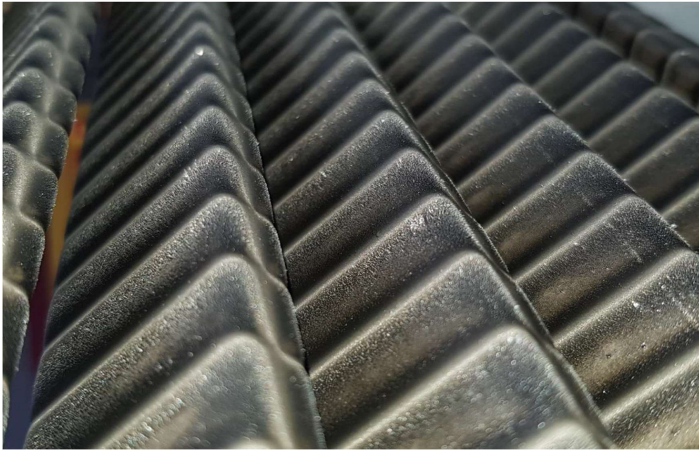
Mag-Shield from hydraulic tank of EX5600 with long-term contamination problems.
