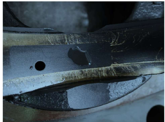
Scoring present on main pump components caused by contaminated hydraulic fluid, prior to Mag-Shield Installation
