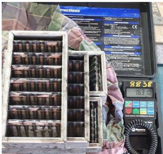
MAG-SHIELDS® weigh 16.31kg after 5180 hours of normal operation.
