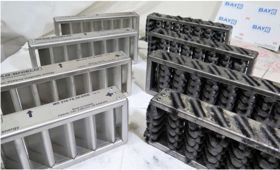
Side-by-side comparison of new Mag-Shields to those that were removed from the CAT 777D post torque converter failure. All the particles on the dirty Mag-Shields were prevented from continuously circulating through the system.
