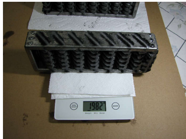
One of four Mag-Shields recovered following the torque converter failure, indicating that 437 grams of material was captured.
