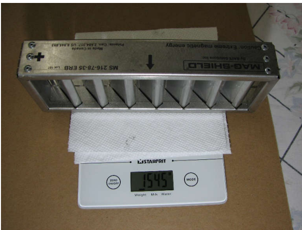
A new Mag-Shield weighs 1.545 kg.
